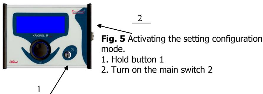
**Fig. 5** Activating the setting configuration mode.
