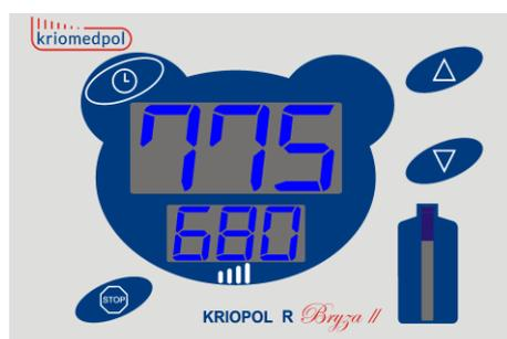
**Fig. 6** Top setting adjustment (current value: 775, stored value: 680).
